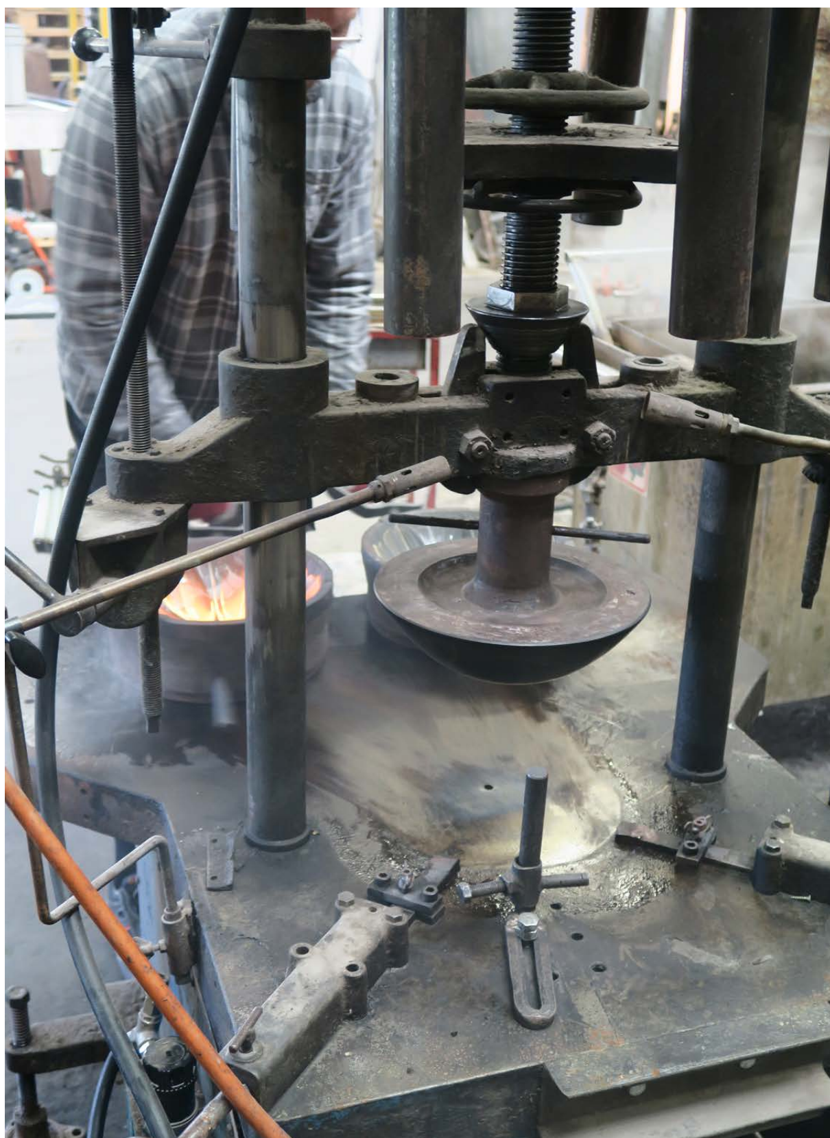
Here are the two guide plates that are anchored to the press table.
