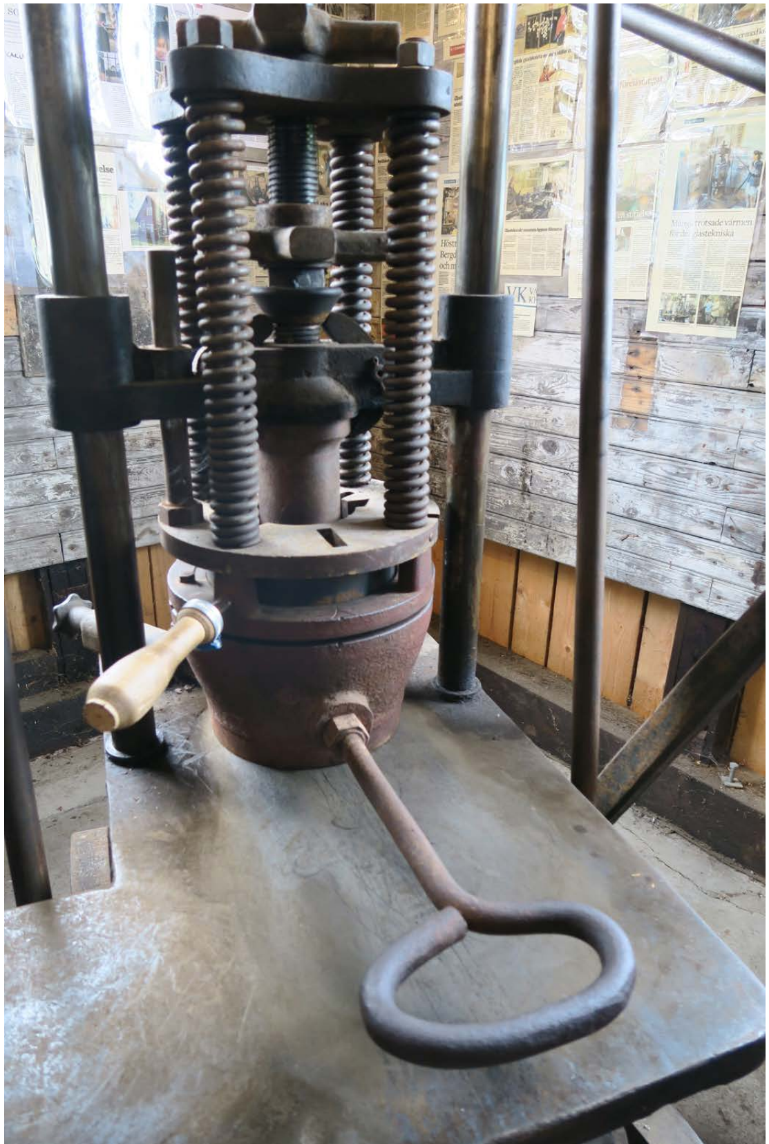
Here the upper edge of the mould is in place but the plunger is not yet pressed into the mould.
