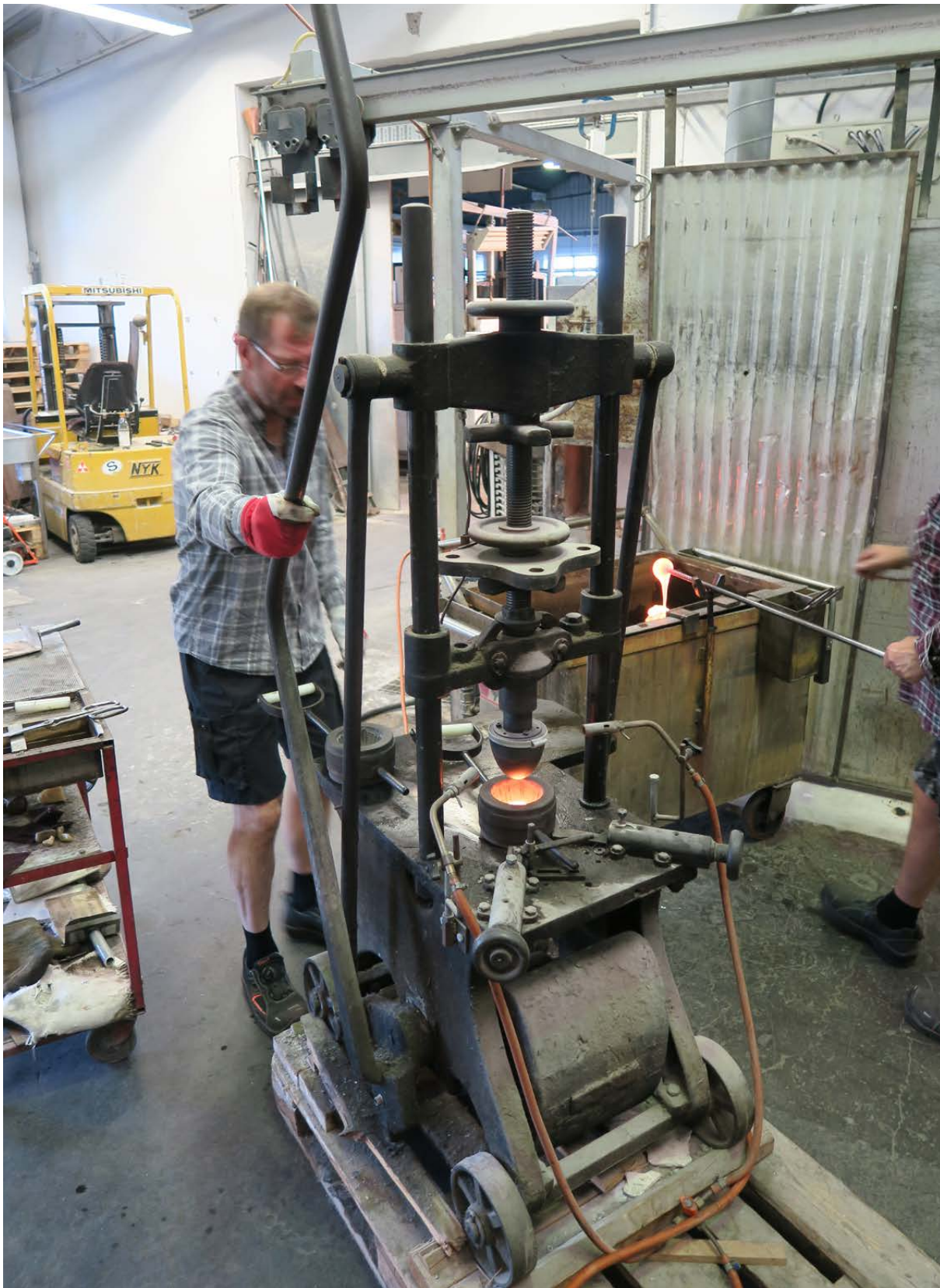
The small bowl uses a smaller glass press from the second half of the 1800s, which is anchored to a pallet. It is completely hand-powered. Tommy Karlsson is the presser in the picture.
