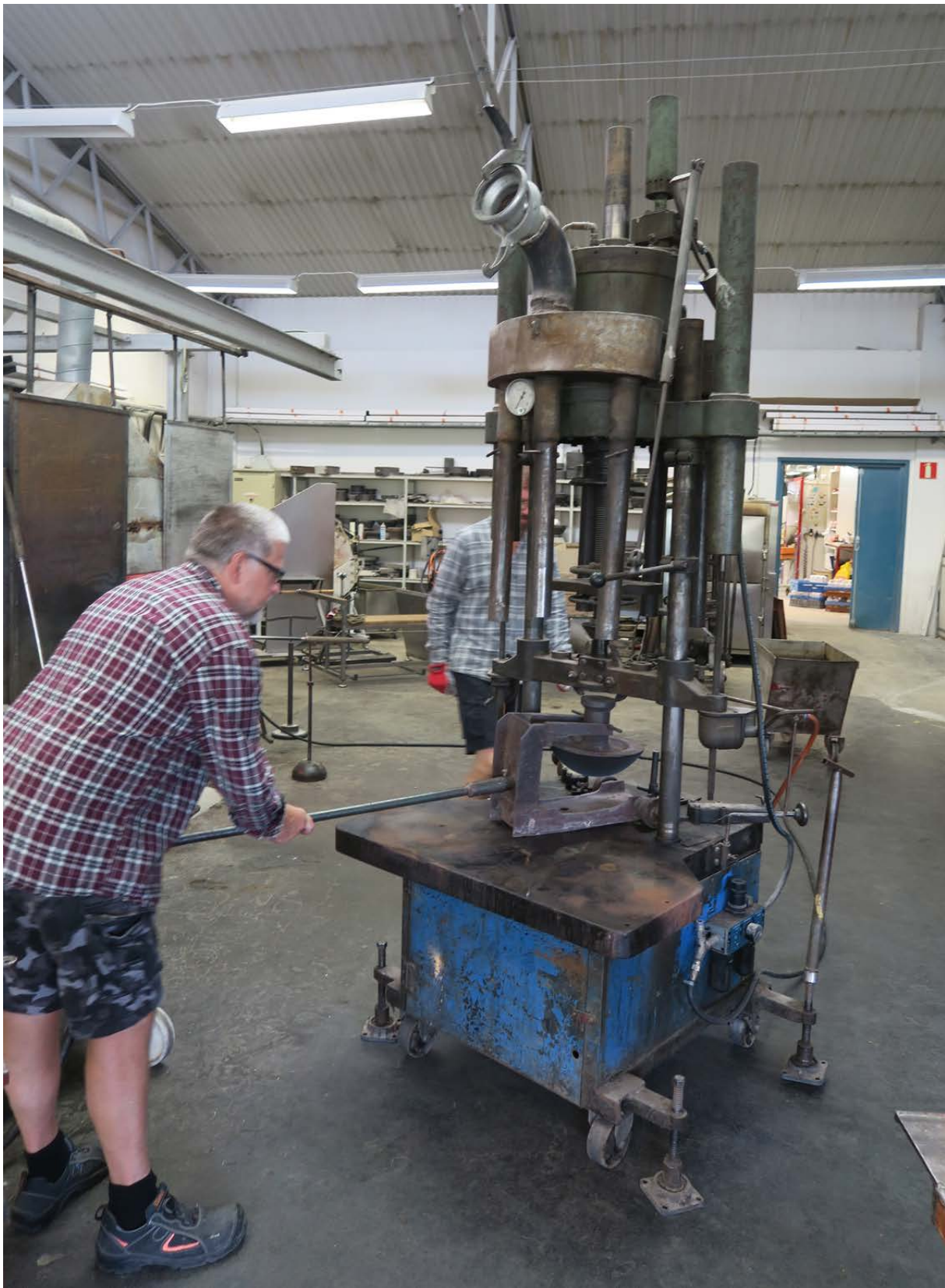
The plunger hangs on a stand that is allowed to slide out over the press table. Two grip claws from the press hold the plunger in place and then the stand can be removed. This press is from the middle of the 1900s.
