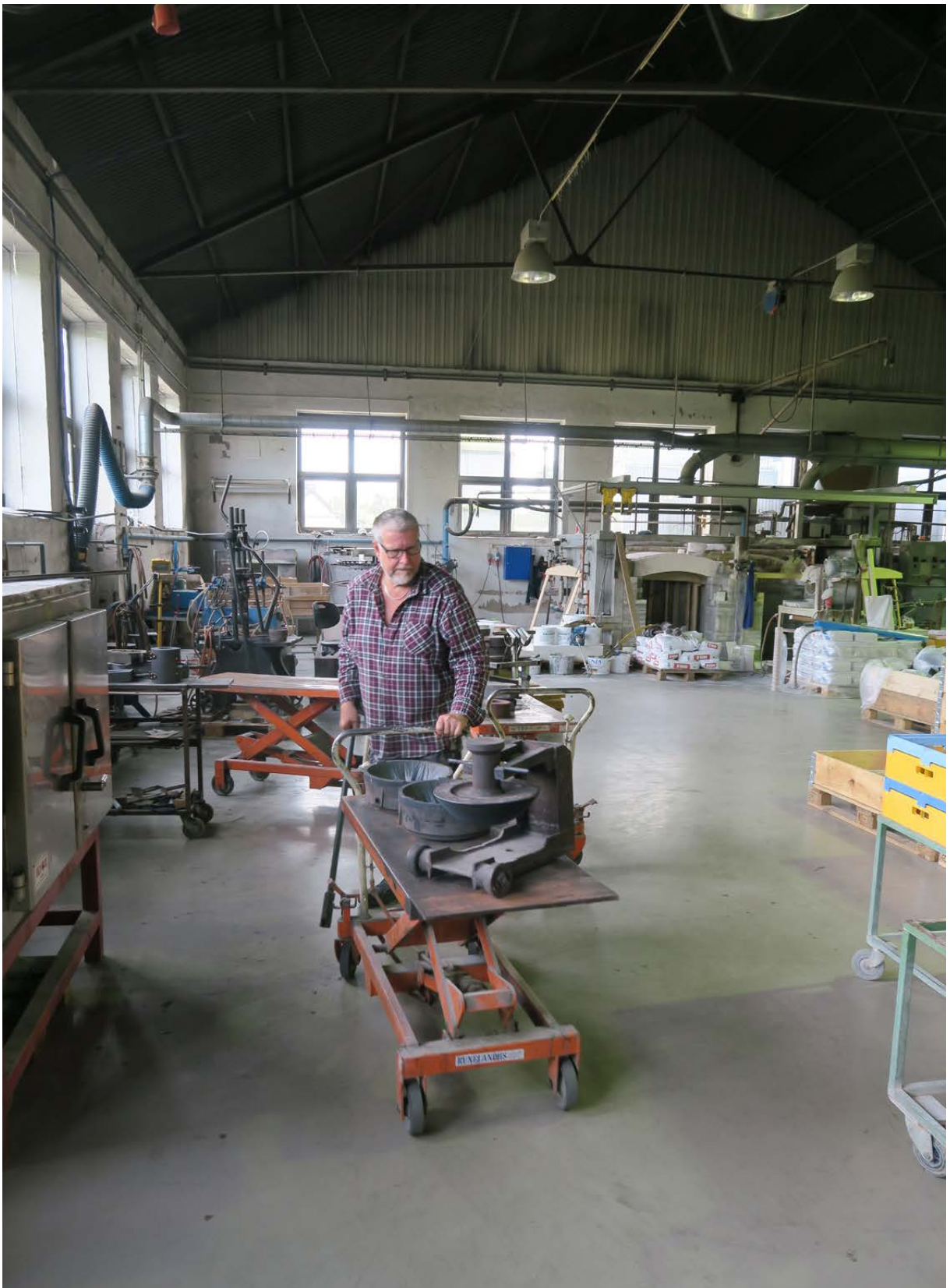
From the annealing kiln to the left of the picture, Erik Boden has taken out two moulds and a plunger on its dolly to be moved to the press. They have a temperature of 480 degrees Celsius.
