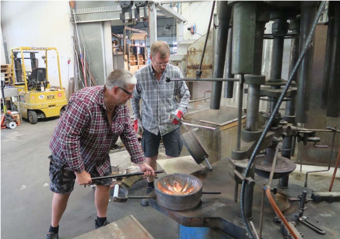
The cooled bowl is allowed to slide out of the mould and is caught by the carrier.
