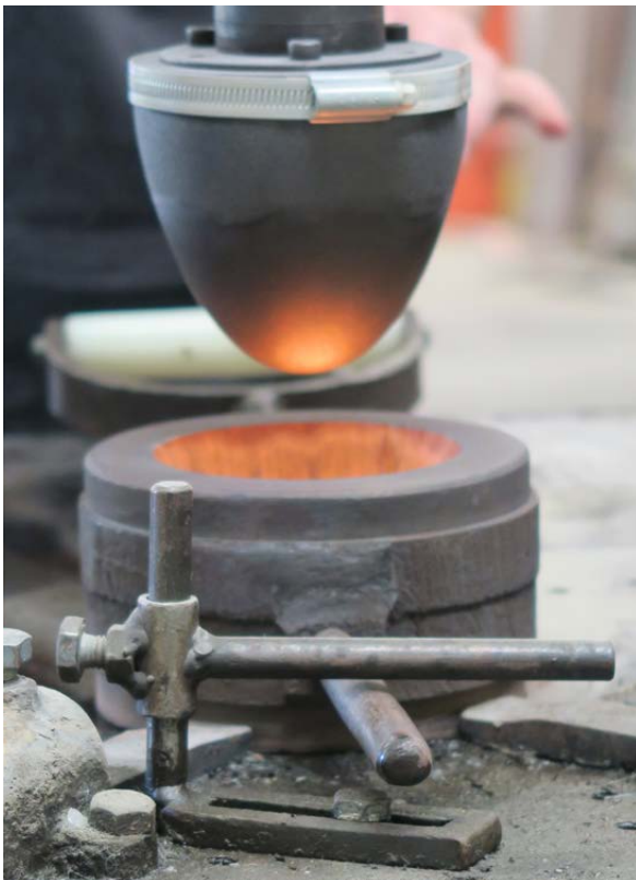
A detailed image of the plunger, which in this case is made of graphite. The plunger is turned at the factory from a cylinder-shaped blank.
