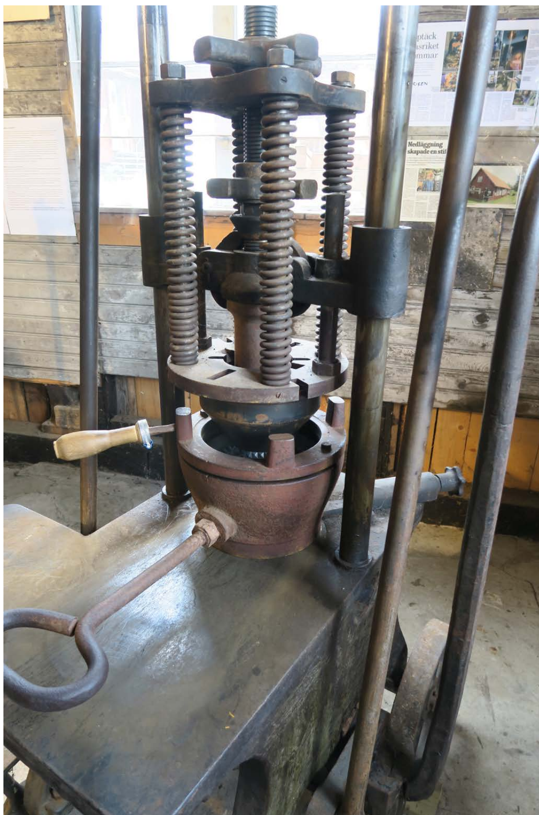
A press for moulds with a ring that has an external spring load. Here the plunger is not yet pressed.
