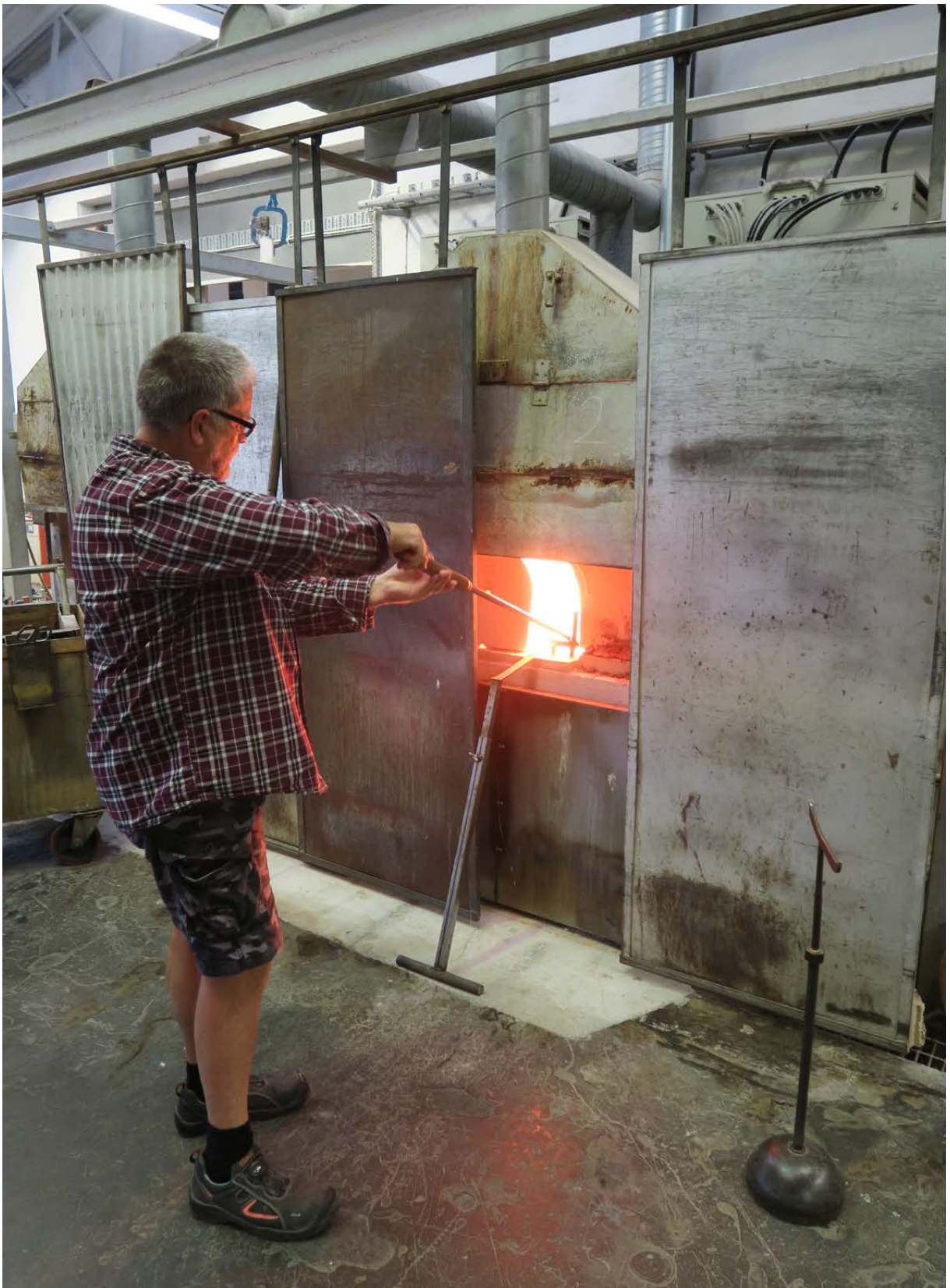
The glass mass is heated to a temperature of 1090 degrees Celsius.
