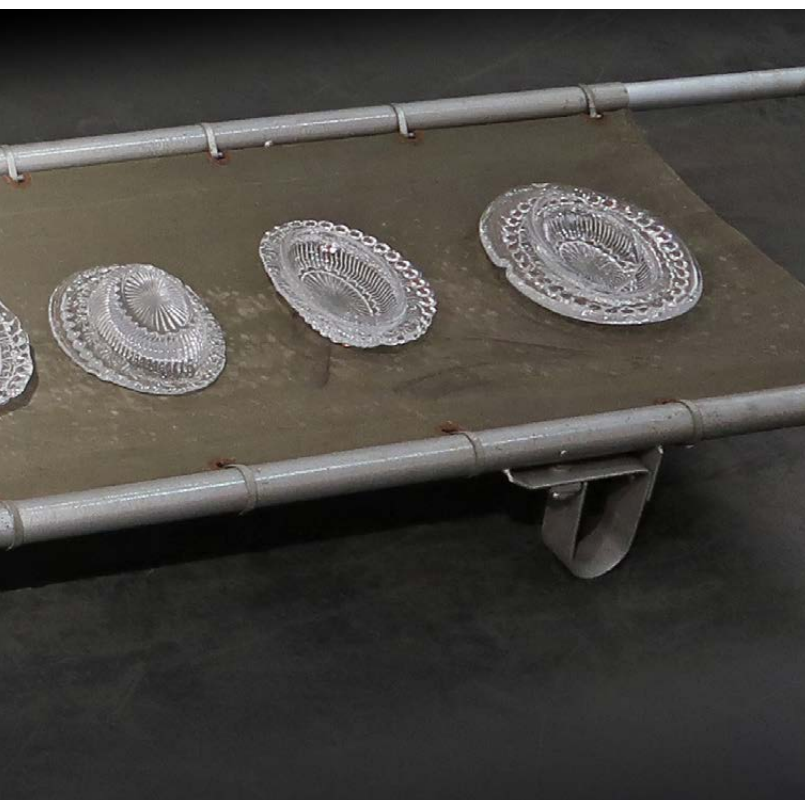
The Glass Factory shows a temporary exhibition with some freshly pressed bowls from the experiments with pressed glass that have been carried out. The picture clearly illustrates how critical the right amount of glass mass is for the end result. Photo: Susann Johannisson.
