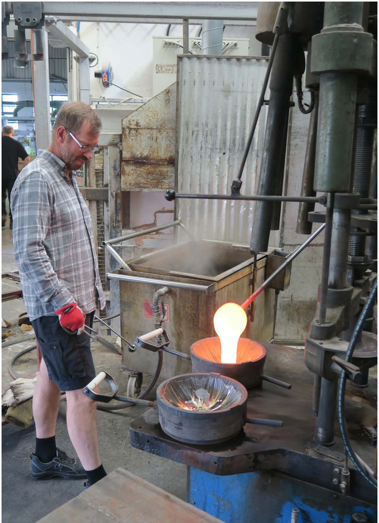
The presser waiting for the glass mass to flow into the mould.
