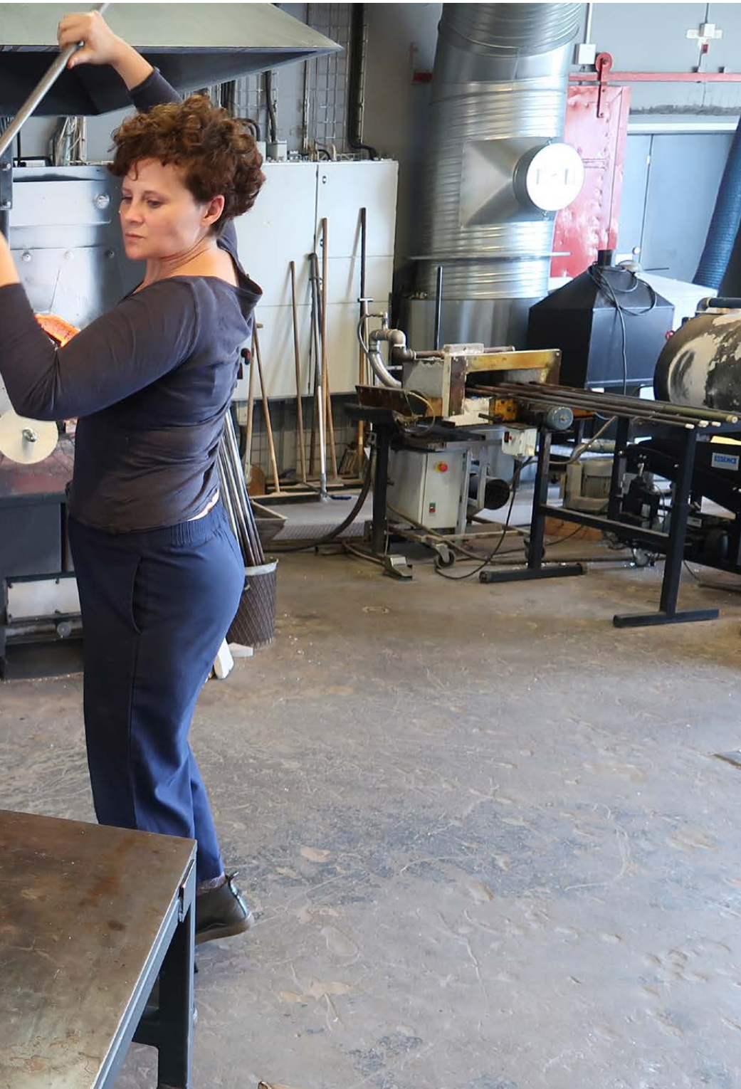
A workshop at The Glass Factory, Boda Glasbruk, September 14, 2019. Glassblower Peter Kuchinke attempts here to make a pressed glass dish where the mould has a ring, assisted by glassblower Tillie Burden. In the picture we see Peter cutting an appropriate amount of glass mass. The mould is divided into three parts, one bottom, one centre part and one ring. Photo: Susann Johannisson.
