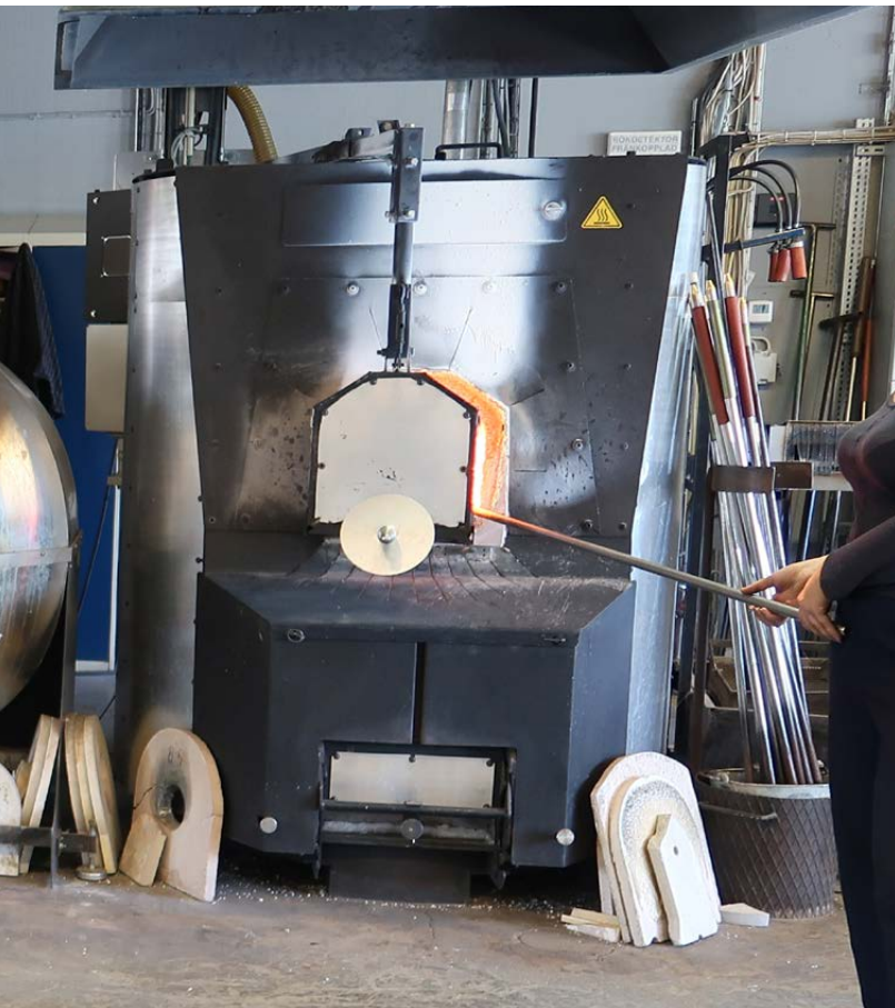
Here we see how Peter turning the mould to take out the glass dish. Photo: Susann Johannisson.
