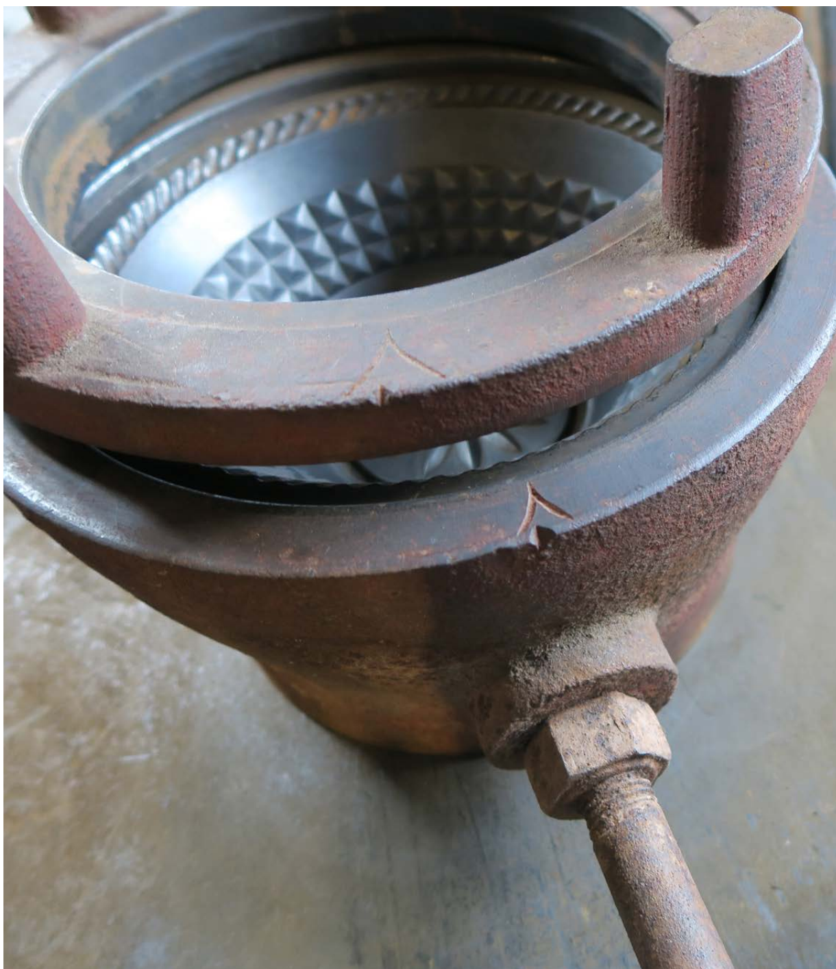
The ring is fitted with two guiding notches, in this case, two V's that match up.
