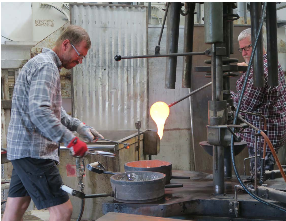
The presser has just cut the desired amount of glass mass.
