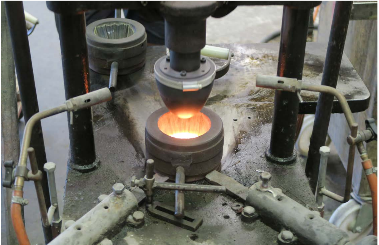
The small press does not have a mould of cast iron but of graphite. The plunger is warmed with gas.
