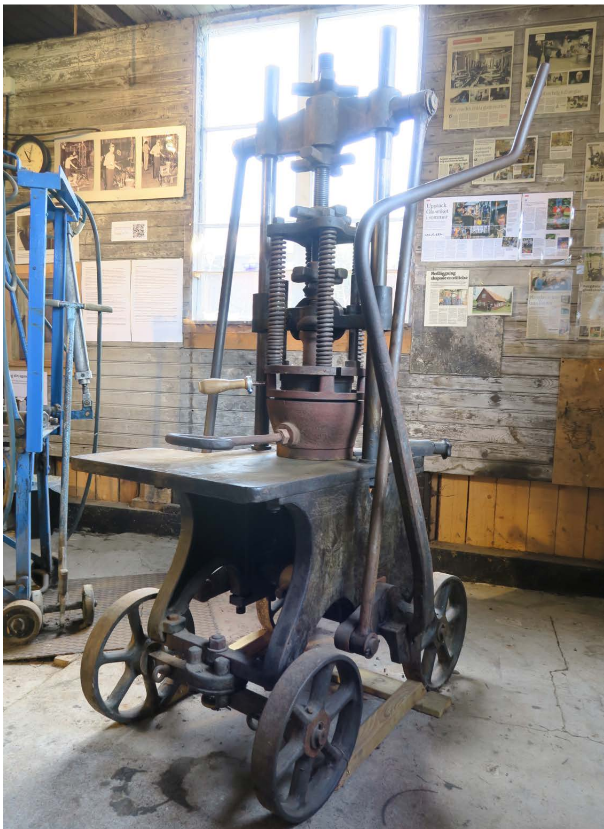
At Bergdala Glass Technology Museum, this glass press is from the second half of the 1800s. This glass press demonstrates how a press with mould and ring works.
