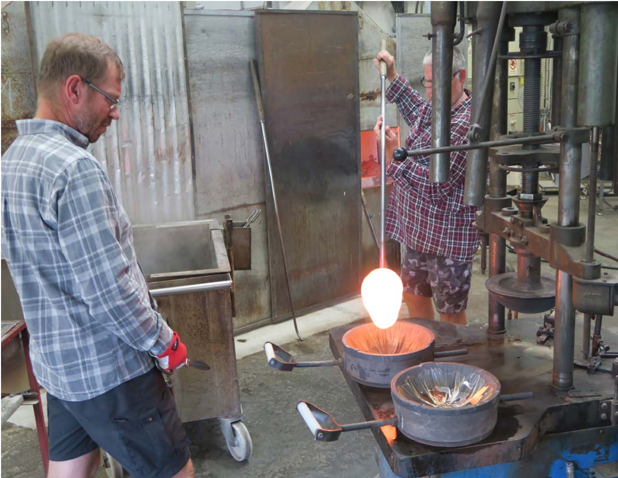
A gatherer takes an appropriate amount of the molten glass from the furnace on a gathering ball and goes over to the press. The gatherer holds the glass mass over the mould.
