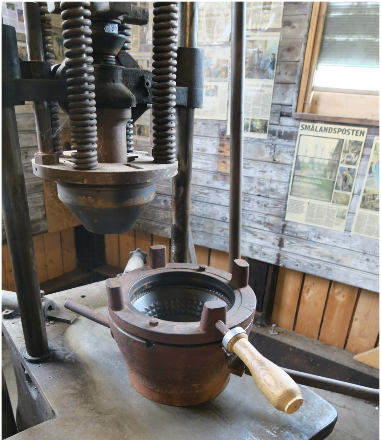
Here the ring has been fitted into the mould.
