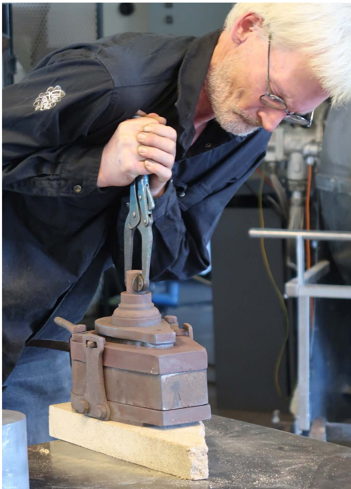
Peter presses the preheated plunger into the mould by hand. Photo: Susann Johannisson.
