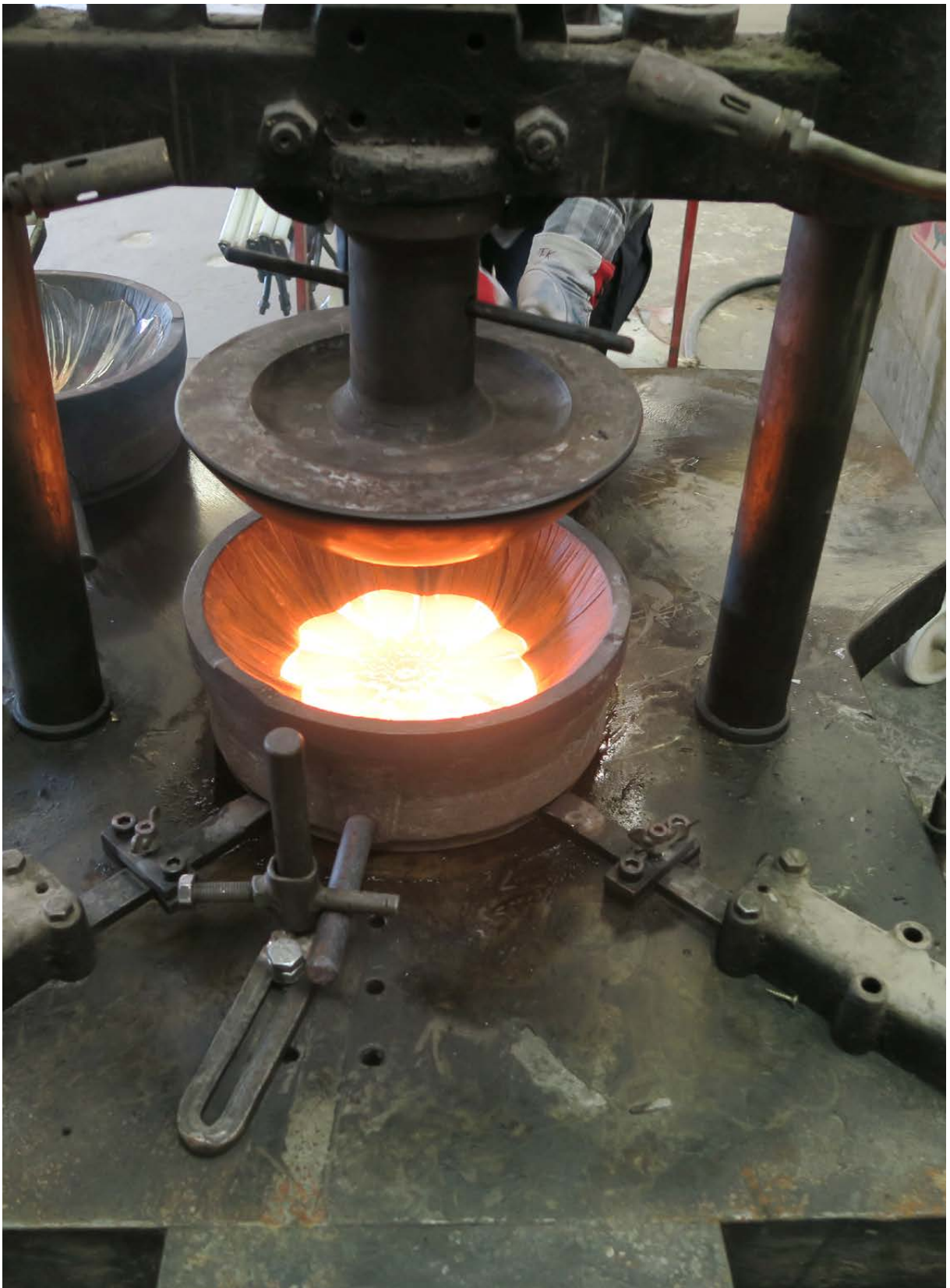
The mould is placed underneath the plunger. The presser is ready to push a pedal which presses the plunger down with compressed air.
