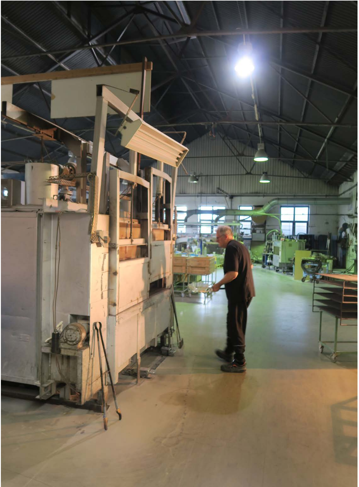
To the left of the image is the annealing kiln. The carrier has just moved a freshly pressed glass bowl to the annealer.
