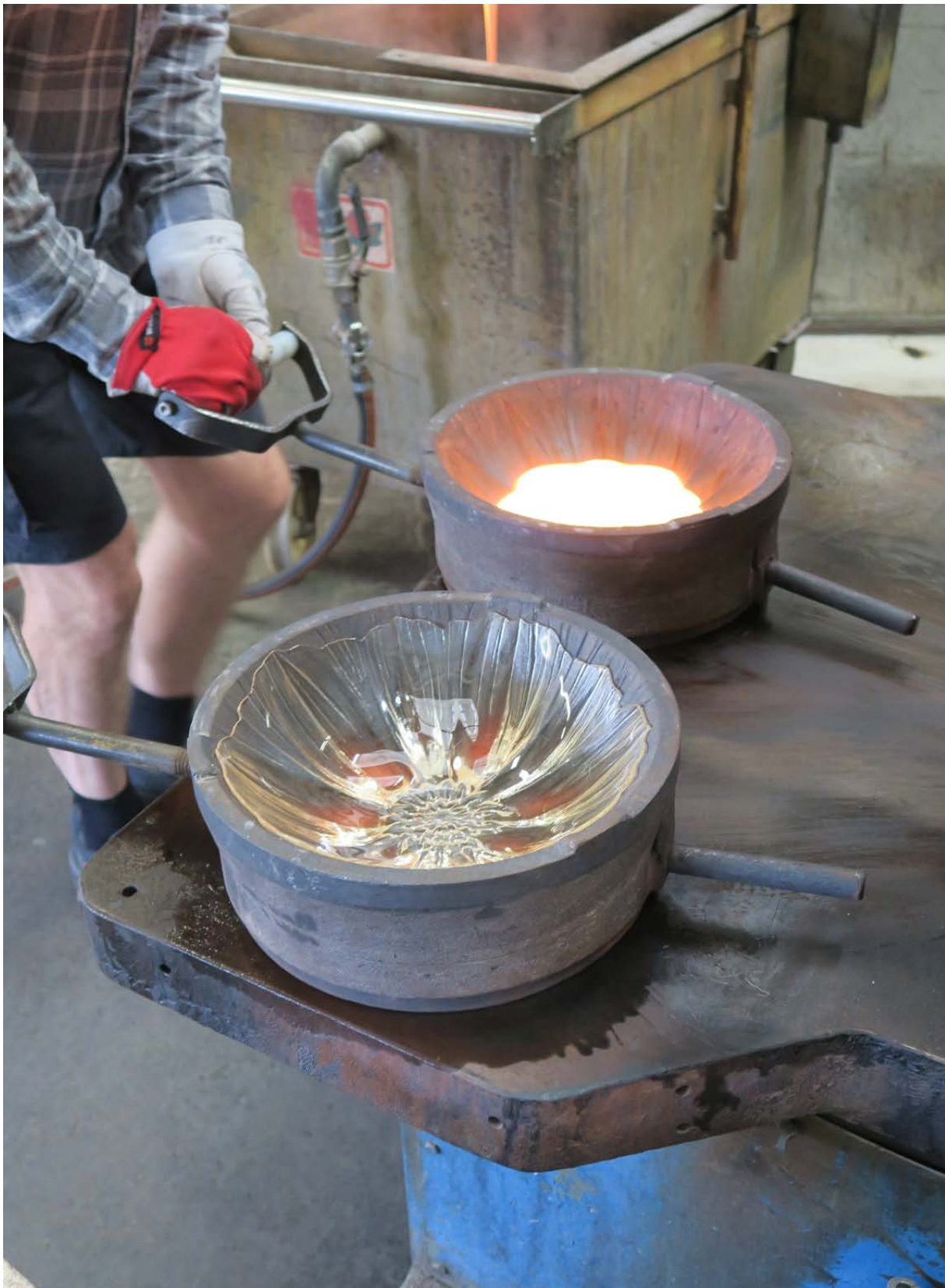
In the foreground is a mould with a pressed glass bowl ready for cooling. In the background, the mould with glass mass is on its way to being pushed into the press.
