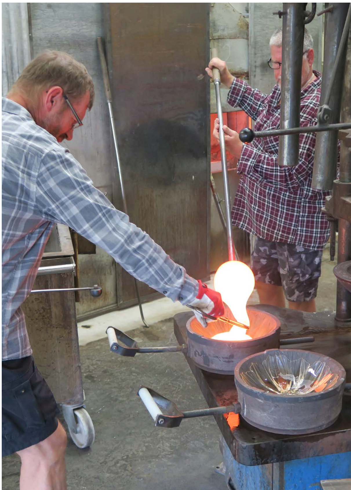
The presser cuts the glass at just the right moment to get the desired amount of molten mass into the mould.
